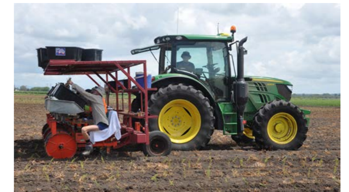
Figure 4.12 – Mechanical planting of tea tree seedlings into newly prepared paddocks. Soil preparation and calibrated planting systems ensure uniform establishment across commercial plantations.
