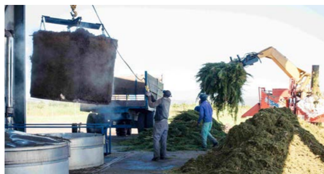
Figure 5.2 Loading tea tree material into the distillation vessel.
