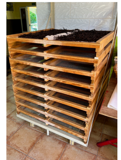
REUNION Drying rack where the cured beans are held to complete drying
