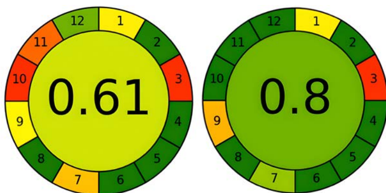
FIGURE 6. AGREE graphics obtained for RP-HPLC-PDA (left) and SFC-PDA (right) methods for the analysis of oxygen heterocyclic compounds in citrus EOs.
